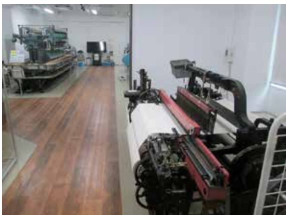
Figure 2. Dynamically drivable textile machines. Left back is the non-stop shuttle change Toyoda automatic loom type G and right front is the Nissan automatic silk reeling machine Type HR-2. Photo S. Tanabashi.
